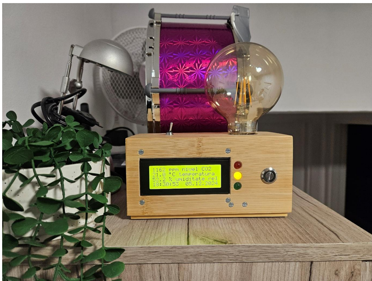
ALEA HomeMonitor device showing live CO 2 concentration, air temperature and relative humidity
